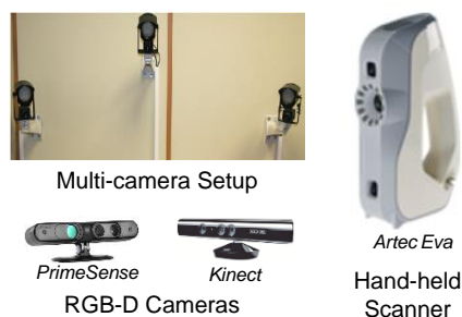
Figure 5.7: Multi-camera setup (Hontanilla & Aubá, 2008), RGB-D cameras (Gaber et al., 2015; Vinokurov et al., 2015) and 3D hand-held scanner (Özsoy et al., 2019) used in 3D facial motion capture systems.
