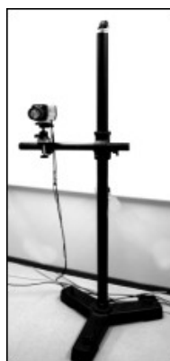
Fig. 40: FLIR A40 IR camera on laboratory stand.
