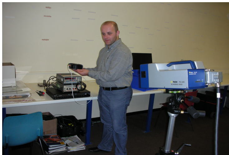
Fig. 79: The laser vibrometer measuring the vibration magnitude from the vibration device, the posture for the real objective test (holding the device with all fingertips).
