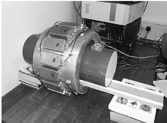
**Figure 5.** The MIT system imaging a simulated oil/gas/water mixture in a cylindrical pipe phantom.
