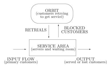
Figure 1. General structure of a retrial queue
