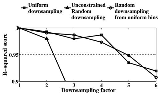
Figure 7: R-squared score for uniform downsampling, random downsampling from uniform bins and unconstrained random downsampling for an effective downsampling factor varying from two to six.
