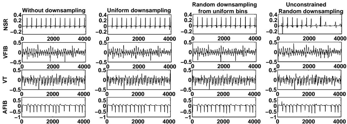
Figure 6: Reconstruction of 4 ECG signals in Figure 3a from one fifth of their respective measurements.
