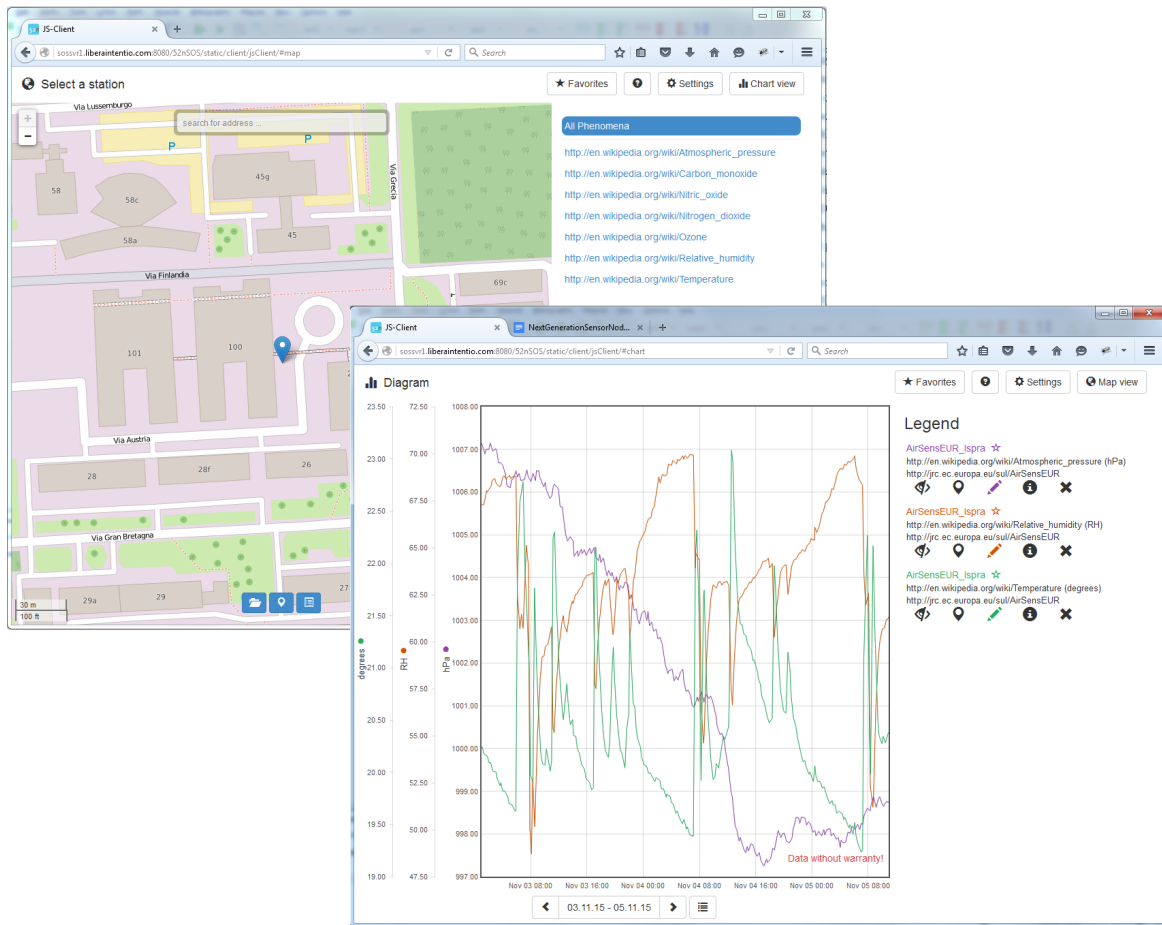
Figure 5. User interface of the 52° North SensorWeb client, loaded with AirSenseEUR data.
