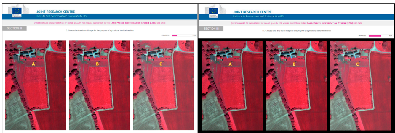
Figure 2. Two questions concerning brightness and contrast using the same images but presenting them on different background colors—white (question 3, Left ) and black (question 11, Right ). The orthoimages displayed have the following properties (brightness and contrast): A (−30, 0), B (0, 0) and C (15, 0).
