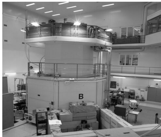
Figure 6.12.1: TRIGA MARK II Mainz: 100 kWth steady state; 250 MWth pulse mode
