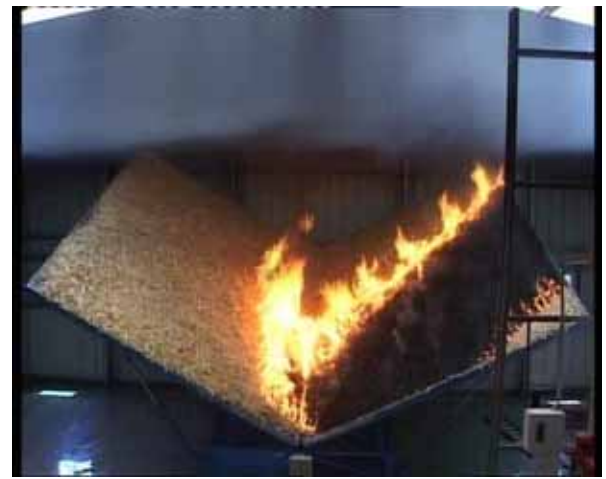
Figure 3.4. Sequence of images of fire spread during the first 100 seconds of the test performed at the DE4 of LEIF. The time step between frames is 20 seconds.
