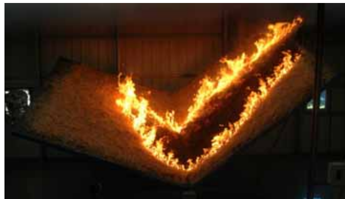
Figure 2.4. Experimental simulation of fire spread during the Guadalajara accident at the large Canyon Table DE4 of the Fire Laboratory of ADAI.
