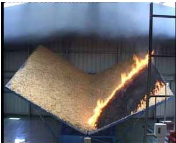
Figure 3.4. Sequence of images of fire spread during the first 100 seconds of the test performed at the DE4 of LEIF. The time step between frames is 20 seconds.
