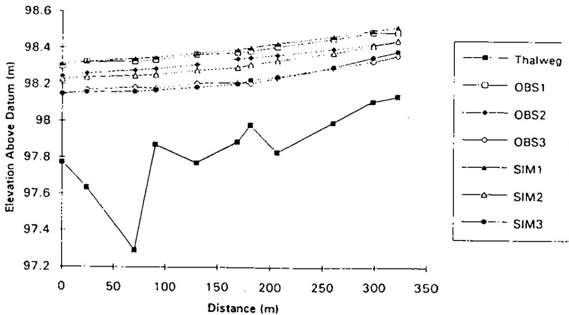
Figure 7: Observed and simulated water surface levels
