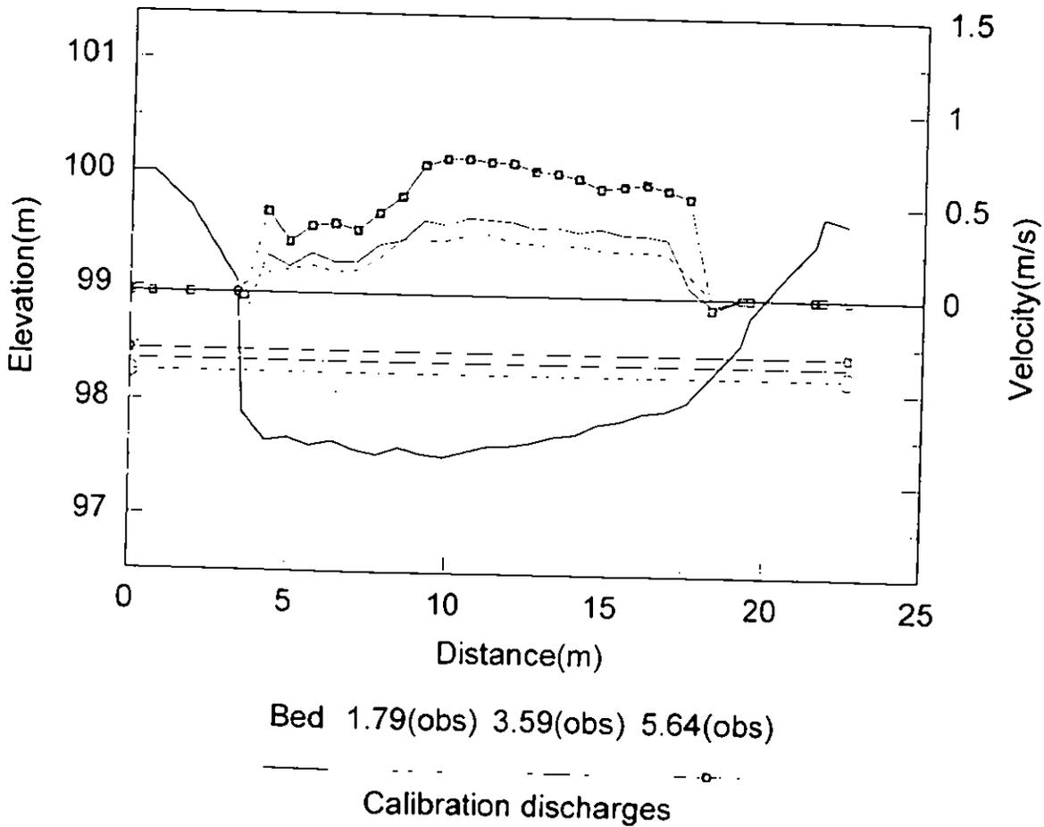
Figure 5: velocity, channel profile and water surface level measurement at three flows
