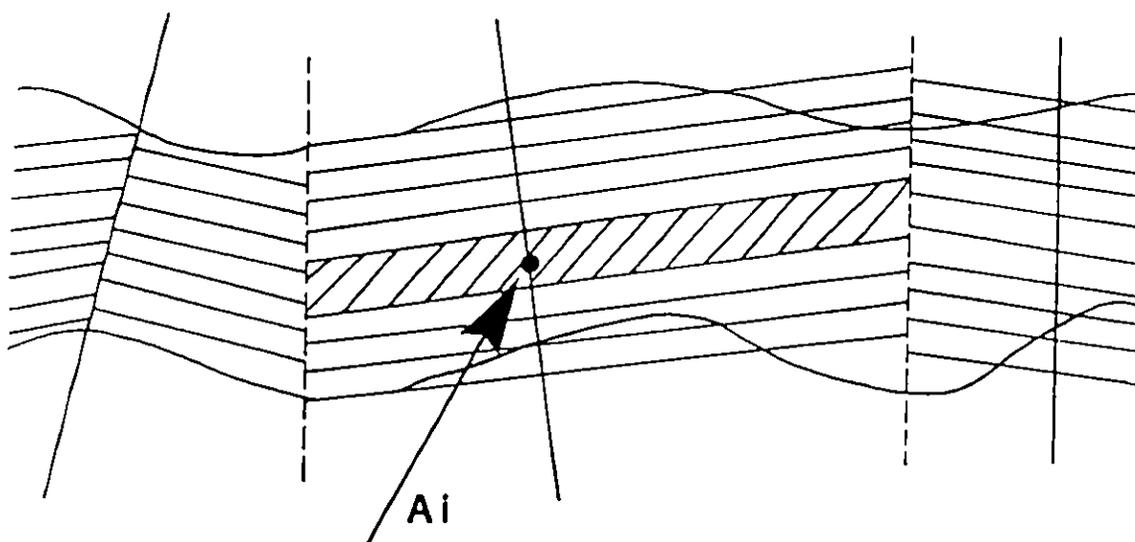
Figure 6: Cells used in PHABSIM calculations
