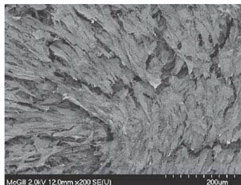
Fig. 5 Surface of the HA coating on PA12C substrate after 15 days of incubation
