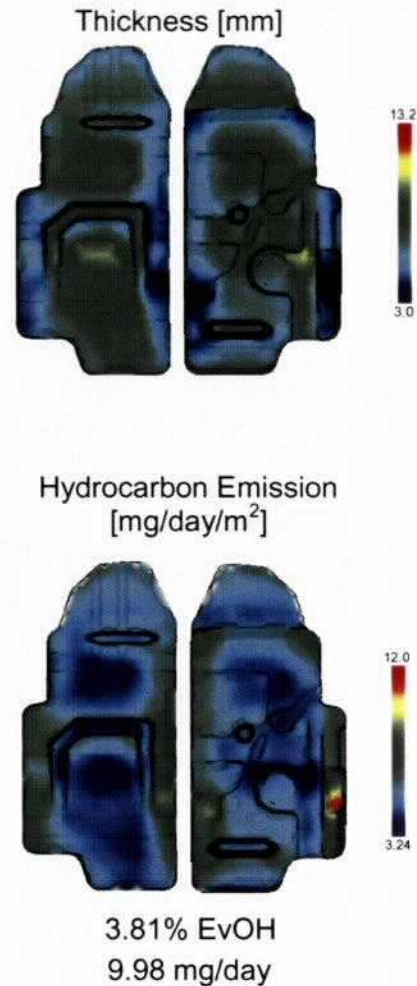
Figure 6. Optimized thickness and hydrocarbon emission flux distributions for the final design after 6 optimization iteration.
