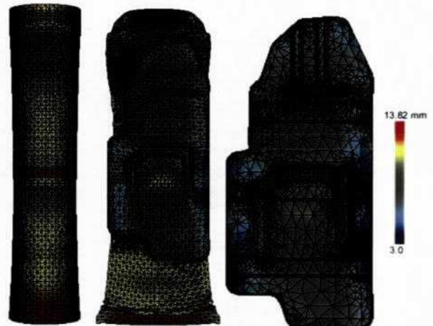
Figure 4. Typical finite element meshes used for the simulation of the extrusion blow molding.
