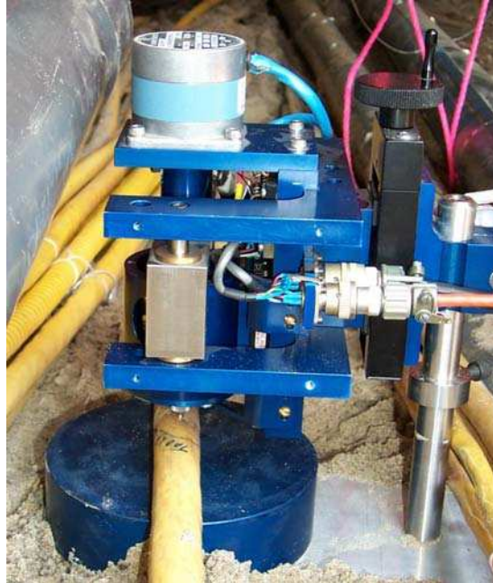
Figure 1 EDST Test Stand Used to Assess Damaged Cables at CRL
