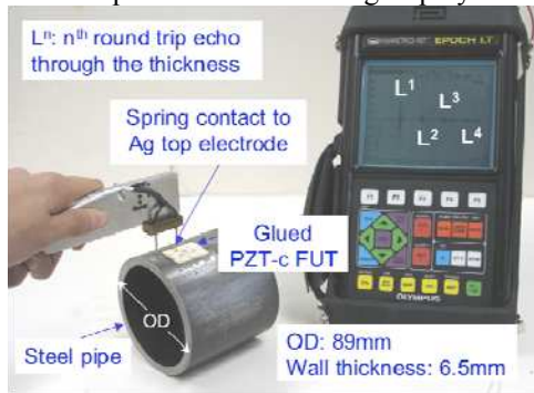
Figure 1. A FUT fabricated on a 75\ \mu\text{m} thick titanium membrane and glued onto a steel pipe with the ultrasonic measurements displayed using a handheld EPOCH LT pulser/receiver.
