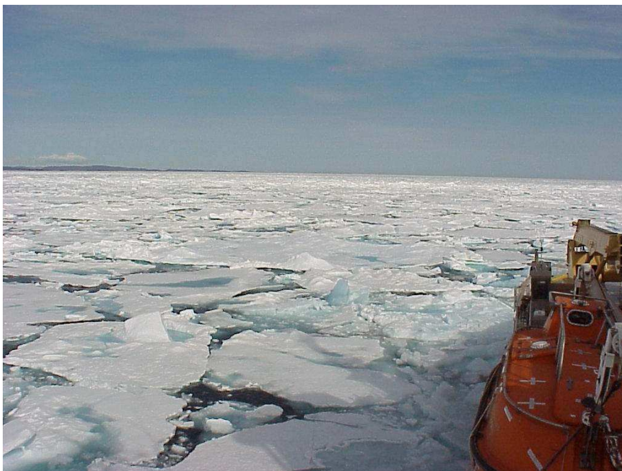
Figure 23: Ice regime with 6/10 TFY, 2/10 SY, 1/10 MY ice observed from the Henry Larsen.
