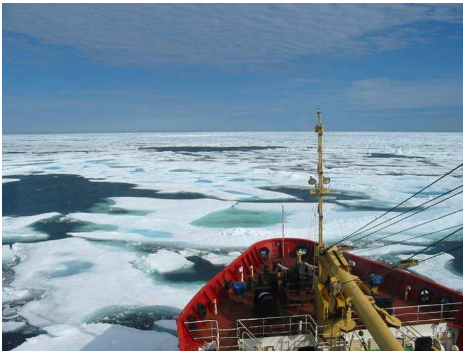
Figure 43: Ice regime with 2/10 MFY, 3/10 TFY, 5/10 MY ice observed from the Sir Wilfrid Laurier.
