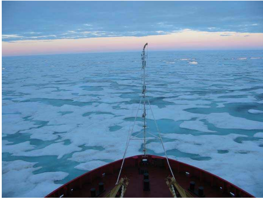
Figure 14: Ice regime with 1/10 FY, 2/10 MFY, 4/10 TFY, 3/10 SY ice observed from the Terry Fox.
