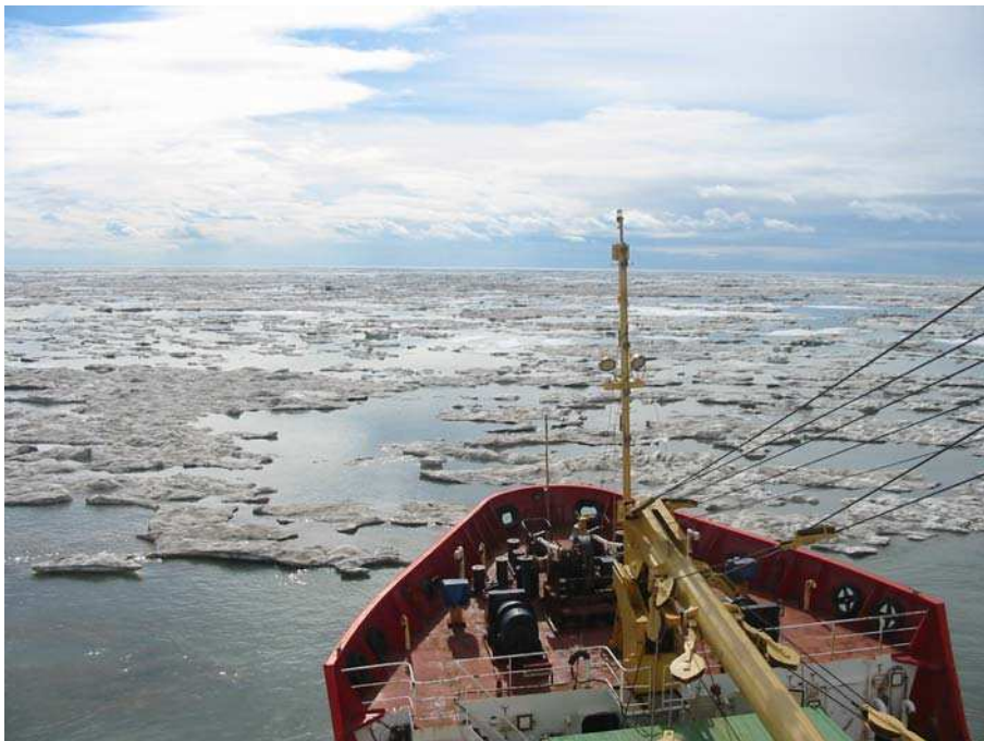
Figure 39: Ice regime with 1/10 MFY, 6/10 TFY ice observed from the Sir Wilfrid Laurier.
