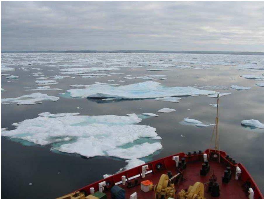
Figure 32: Ice regime with 2/10 MFY, 5/10 TFY, 1/10 MY ice observed from the Des Groseilliers.
