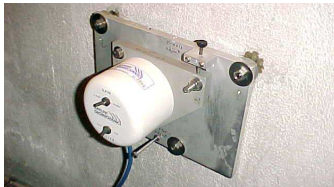
Figure 2 Tiltmeter and mounting plate on the wall of the lighthouse
