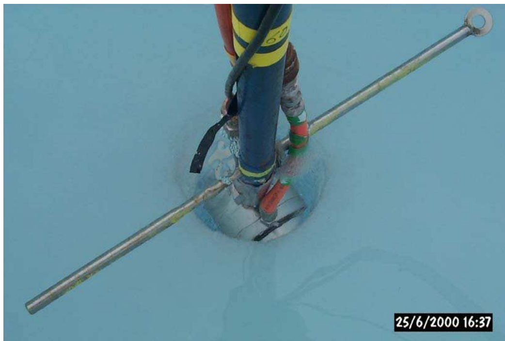
Figure 8: Photograph of the borehole jack in the ice.
