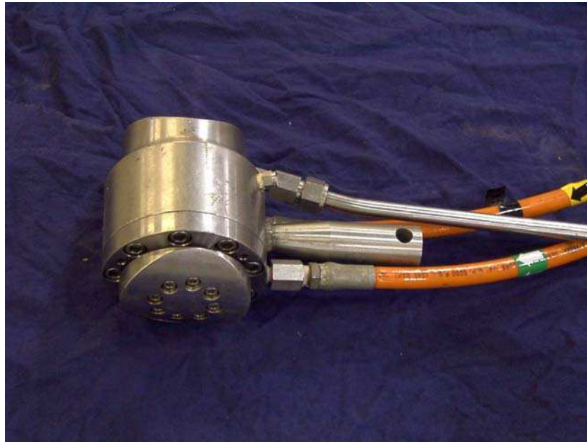
Figure 7: Photograph of the borehole jack
