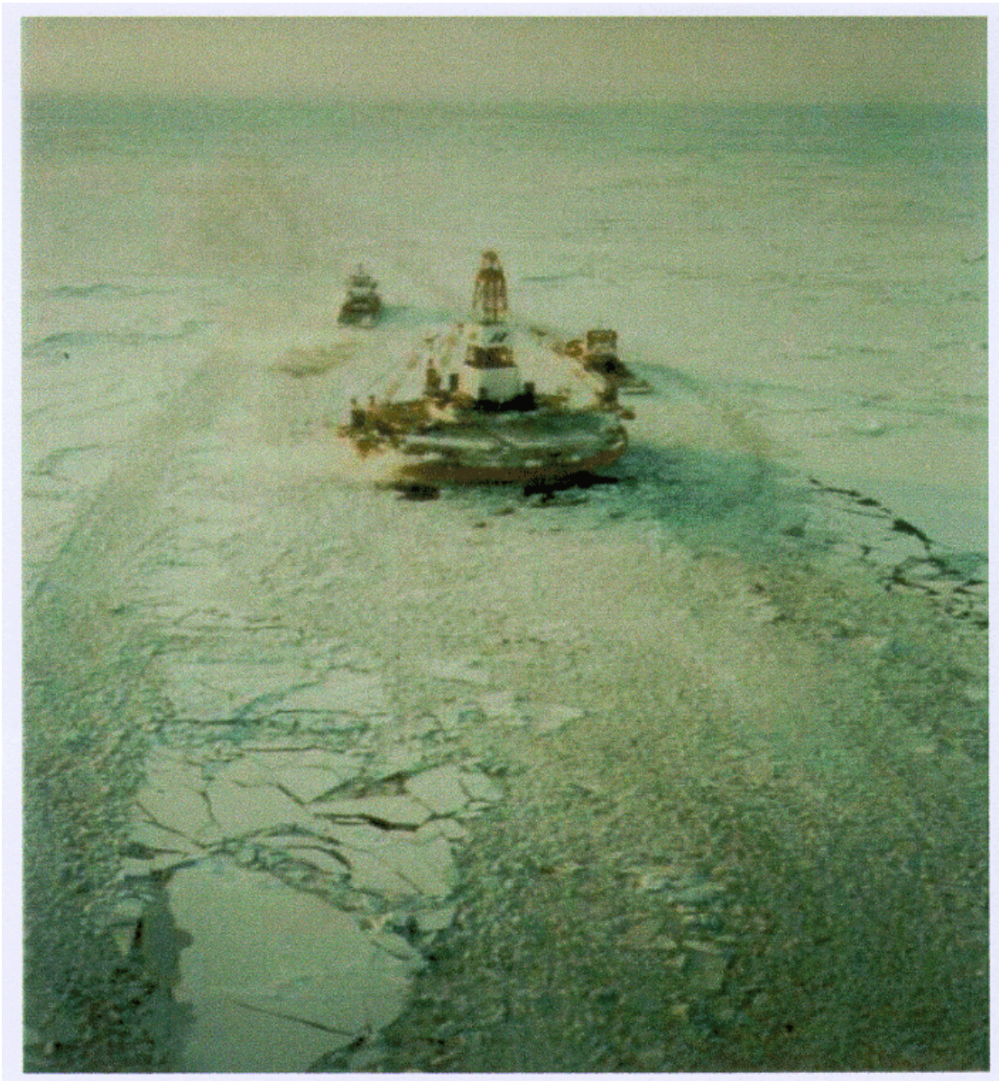
Figure 2.6 This photo shows the Kulluk stationkeeping in late freeze-up/early winter pack ice conditions, with two vessels managing the oncoming ice cover updrift. The ice management technique that was being used at the time involved tandem linear tracks through the oncoming ice cover. The pack ice was near continuous in terms of its concentration, was about 1m in thickness, and had frequent areas of ridging and rubble within it. During the late freeze-up and early winter period, poor visibility conditions caused by frequent occurrences of fog and the long polar darkness, were often an impediment to operations, but were successfully dealt with.
