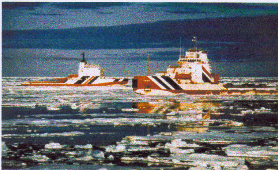
Figure 2.3 CAC 2 icebreakers provided very effective ice management support for the Kulluk drilling vessel. This photo shows two of Beaudril's CAC 2 support icebreakers, the Terry Fox (24,000 HP) and the Ikaluk (14,800 HP)
