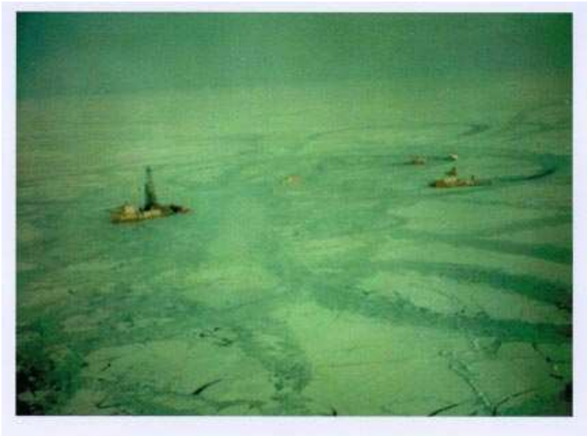
Figure 2.1 Canmar’s drillships were used for exploratory drilling operations in the Beaufort Sea from 1976 until the late 1980’s. Although these vessels were ice strengthened for operations in the Arctic offshore, they were relatively conventional drillships with fairly weak mooring systems ( \approx 100 tonne capacity). Ice management support was quite effective in allowing them to stationkeep in various pack ice conditions. This photo shows the Explorer 4 drillship (which had underwater fairleads) operating in thin moving pack ice conditions during the late freeze-up period, with ice management support vessels working updrift of the drillship. The ice management technique that was being used at the time involved a “circular breaking” pattern.
