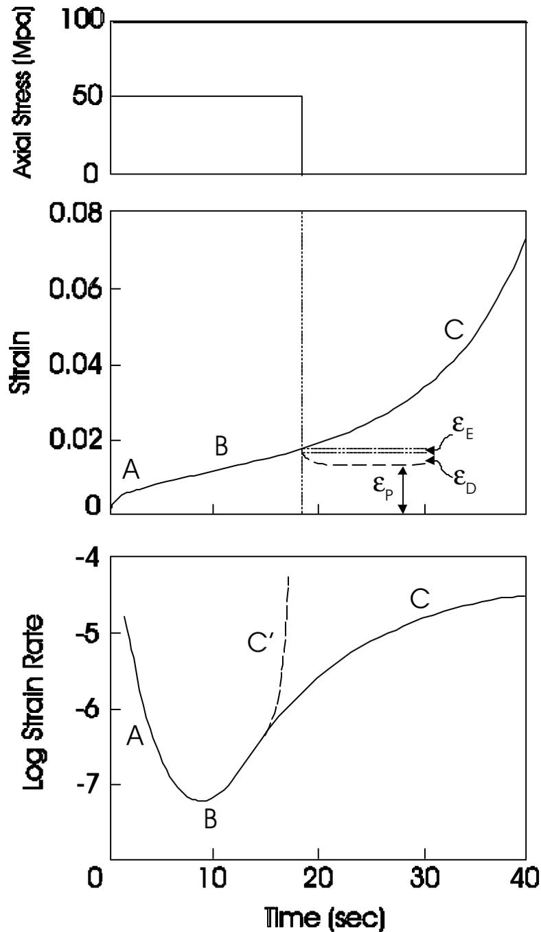
Figure 9: Creep response for freshwater, polycrystalline ice at 55 MPa hydrostatic pressure, 15 MPa axial stress and a temperature of  $-10^{\circ}\text{C}$ . The elastic ( $\epsilon_E$ ), delayed elastic ( $\epsilon_D$ ) and permanent ( $\epsilon_P$ ) component of the deformation are best seen upon unloading the specimen. A: Decelerating creep, B: Minimum creep rate, C: Accelerating creep, C': Run-away behaviour.
