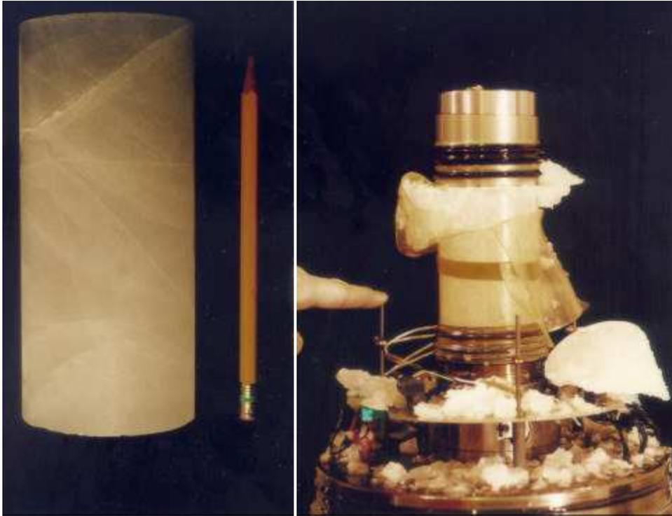
*Figure 27: Example of an unsuccessful test. A planar ‘flaw’ near the top end of the specimen (left) was unable to withstand the axial load on the specimen, leading to immediate collapse. The minimum strain rate was not attained and no data resulted from this test. Pencil and finger for scale.*
