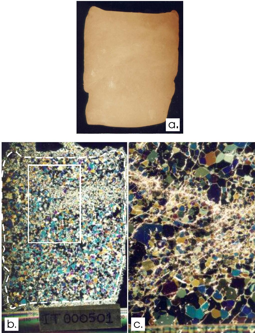
*Figure 25: (a) Specimen of iceberg ice deformed to 31% true strain at a confinement of 50 MPa, -10 °C.. (b) Thin section of whole specimen showing grain refinement along planar zones. (c) Enlarged view of (b) with side (reflected) light, showing the nature of the grain refinement. It consists of new crystals but where fracturing is also present. Scale in mm.*
