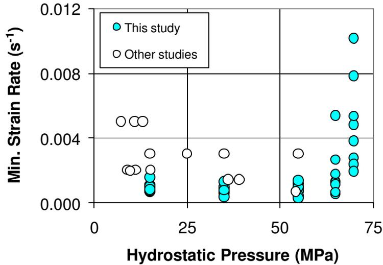
Figure 15: Plot of minimum strain rate as a function of hydrostatic pressure for all tests. The data is corrected for a temperature of  $-10^{\circ}\text{C}$  with the linear regressions in Figure 14. The data from other studies (Jones 1982, Durham et al. 1983, Kalifa et al. 1989, Rist and Murrell 1994 and Mizuno 1998) were obtained from constant strain rate tests (see text).
