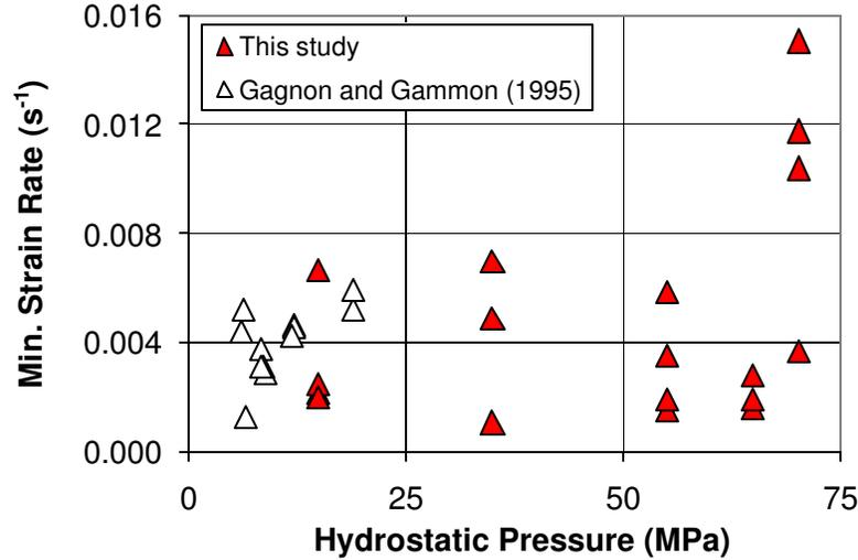
Figure 16: Plot of minimum strain rate as a function of hydrostatic pressure for all tests. The data is corrected for a temperature of  $-10^{\circ}\text{C}$  with the linear regressions in Figure 14. The data from Gagnon and Gammon were obtained from constant strain rate tests (see text).
