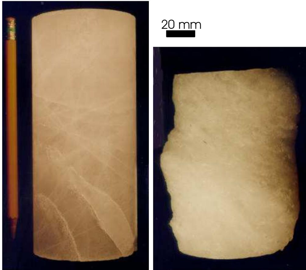
*Figure 23: Ice specimens made from iceberg ice. Left, undeformed; right, deformed to 27% true strain at 7 MPa confinement ( $-10^{\circ}\text{C}$ ). Note the 'flaw' pattern in the undeformed specimen and the inhomogeneous nature of the deformation. The chalky white colour is indicative of widespread microcracking. Unlike the example shown in Figure 27, these flaws did not cause the ice to rupture.*
