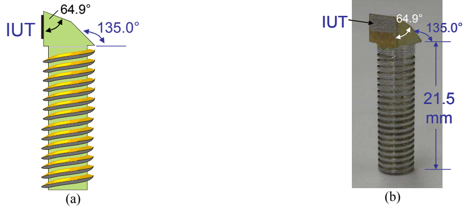
Fig. 3. An Al screw which can generate both L and S waves simultaneously with an IUT located in a plane parallel to the direction of mode converted S wave where \theta = 64.9^\circ . (a) Schematic diagram and (b) actual probe.
