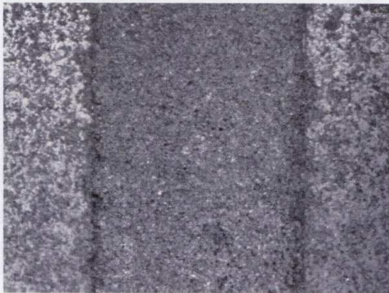
Figure 12 – Wear scar formed during rub-rig testing on the surface of CoNiCrAlY-BN-polyester abrasion coating.
