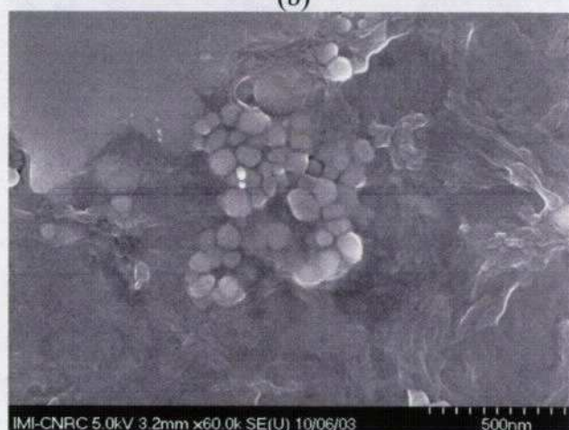
Figure 15 – Different types of nanostructural characteristics found in the cross-section of the HVOF-sprayed nano HA coating of Fig. 14. (a) porous, (b) fibrous [15] and (c) densely packed [15] nanozones.
