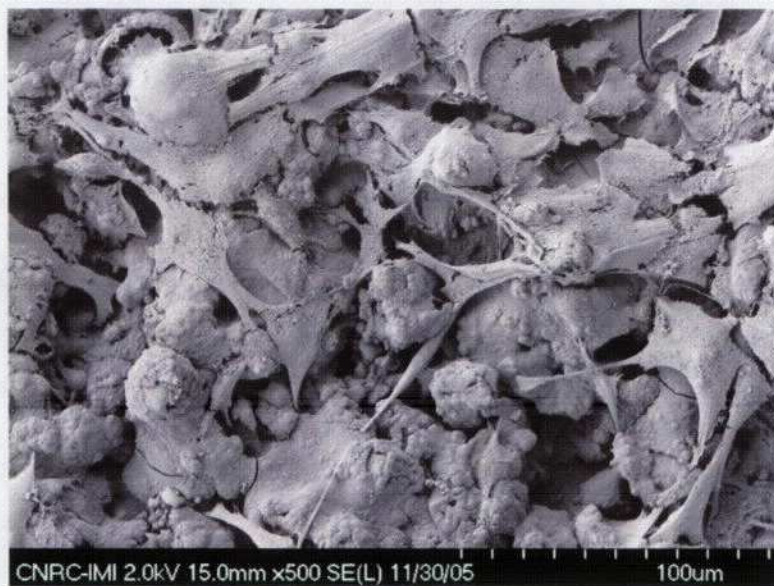
Figure 17 – Osteoblast cell culture (7 day-incubation) on the surface of an APS conventional HA coating.
