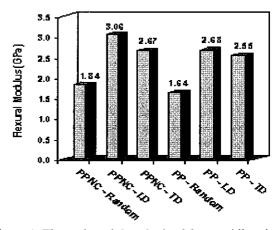
Figure 1: Flexural modulus obtained from unidirectional and randomly oriented plates.
