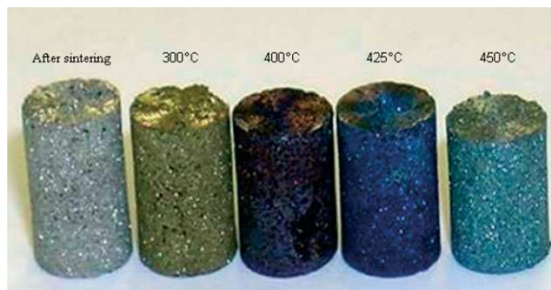
Fig. 8. Specimens after the different oxidation treatments for 1 h in Ar-20%O 2 atmosphere at temperatures ranging from 300 to 450 °C (color: silver, golden, dark purple, blue, light blue-green).
