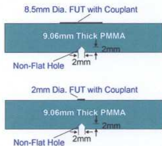
Fig.11. A schematic of a FUT to detect a hole in PMMA plate.
