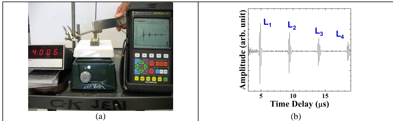
Fig.2 (a) Measurement setup for an IUT made of BIT/PZT composite film at 400°C using an EPOCH LT; (b) Measured ultrasonic data in pulse-echo mode at 400°C.
