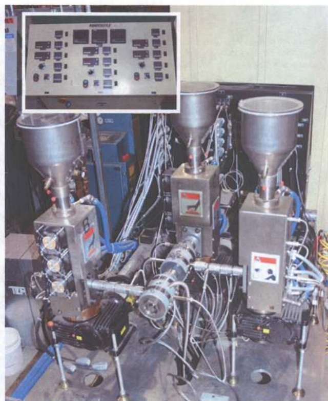
Figure 9. Photograph of the monofilament multilayer spinning set-up designed at NRC-IMI and capable of spinning fibers with up to three coaxial layers of three different materials.
