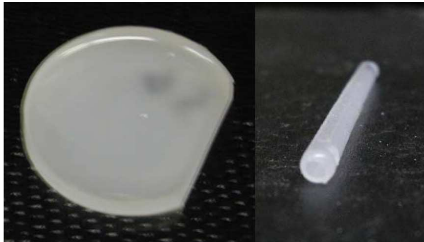
Figure 8. On the left, a disk-shaped phantom of silica microspheres in silicone and, on the right, an artery-shaped phantom of silica microspheres in silicone.
