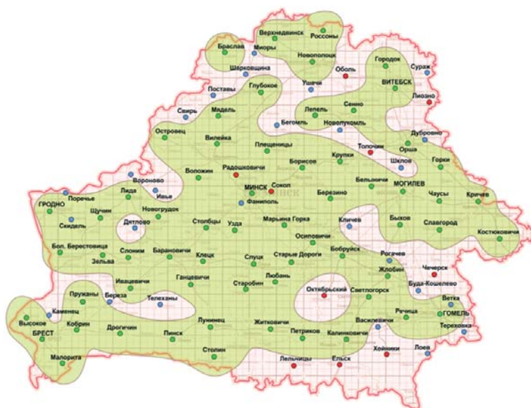
Fig. 1 RTK covering area
