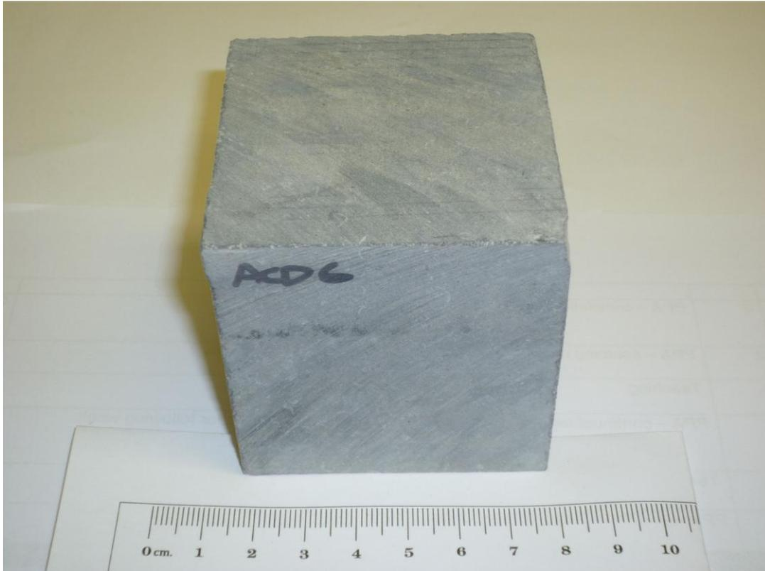
**Figure 4. BGS crushability test cube (60mm). BGS©NERC**
