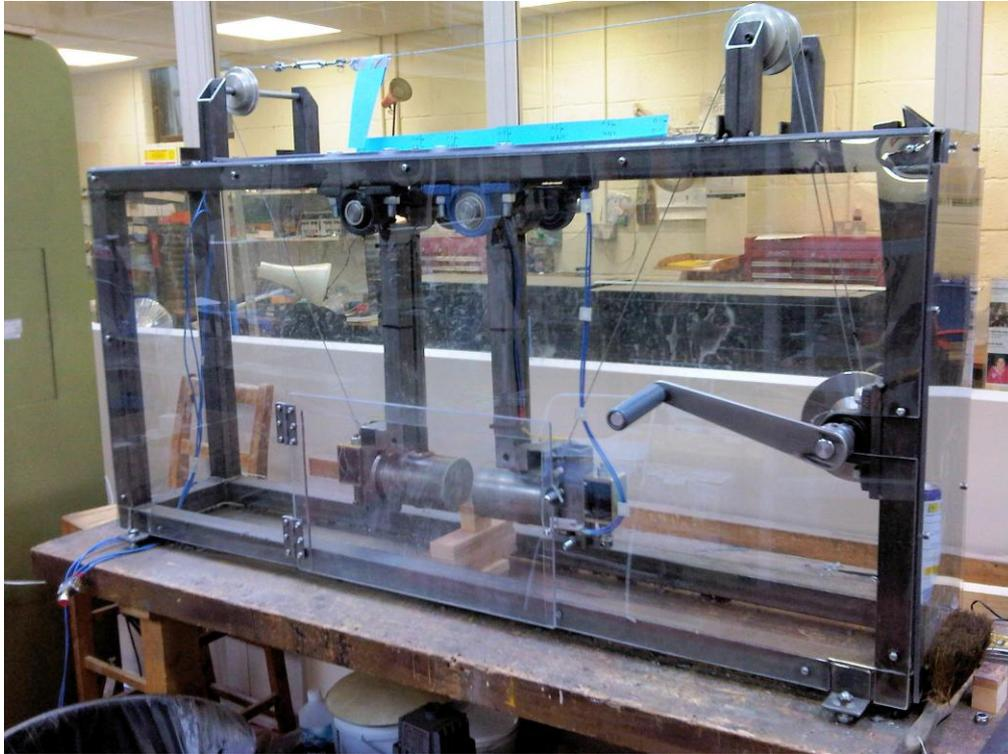
**Figure 2. BGS crushability test device. BGS©NERC**
