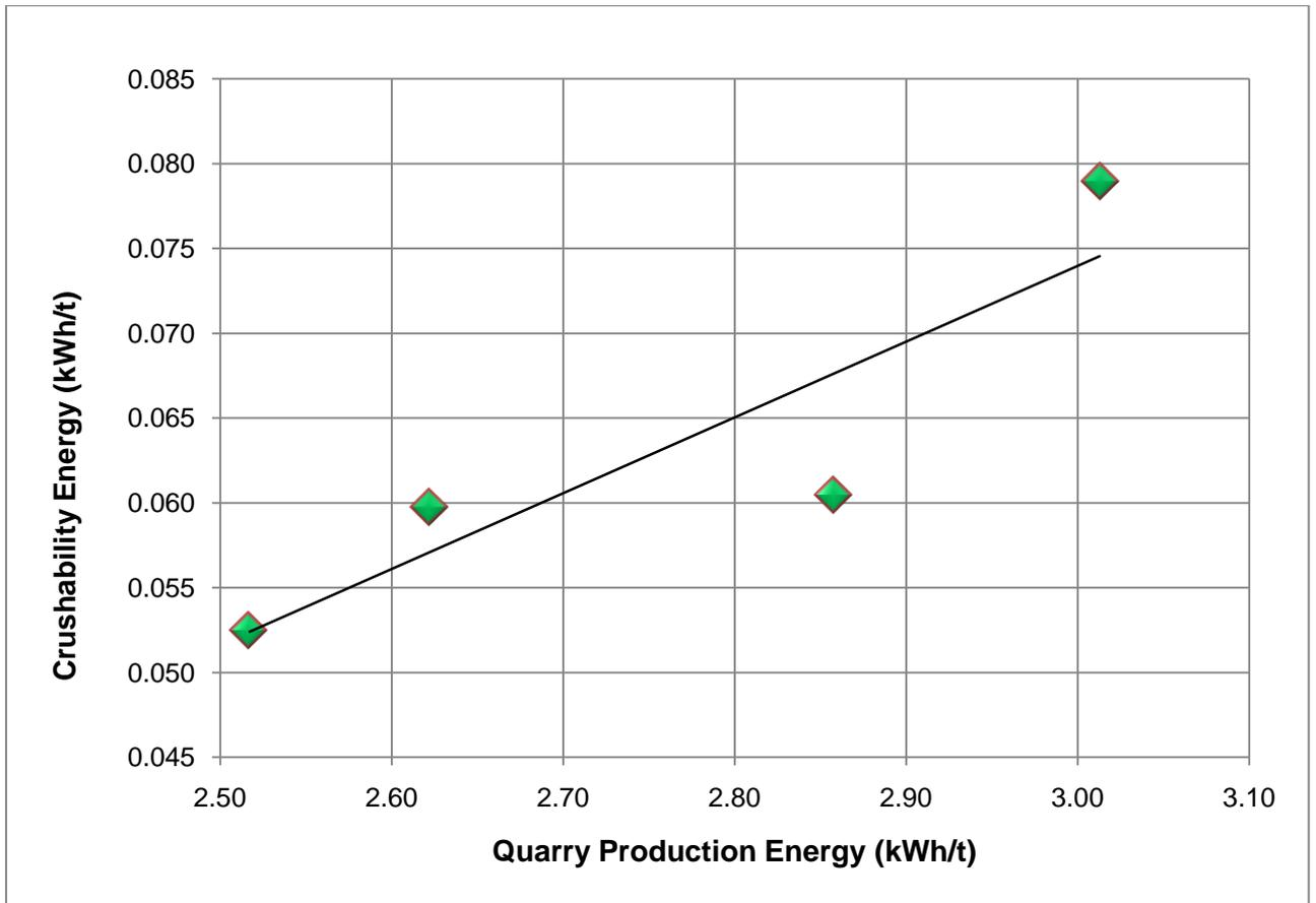
Figure 7. BGS crushability energy and quarry production energy (kWh/t is kilowatt hours per tonne).
