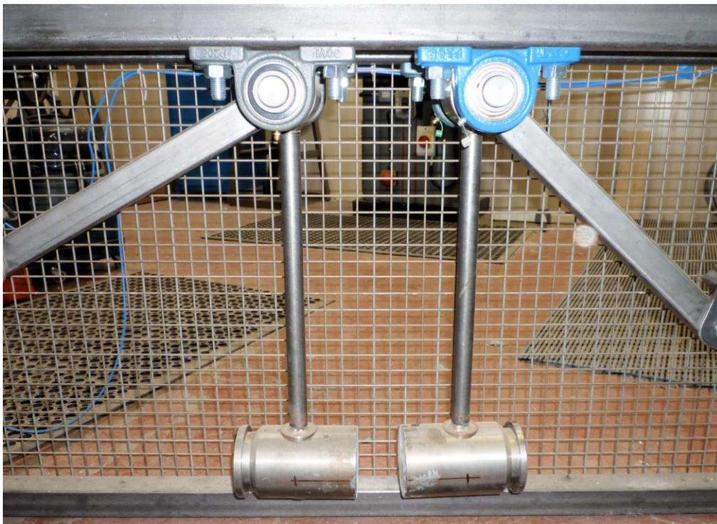
**Figure 3. Close up of BGS crushability test device. BGS©NERC**
