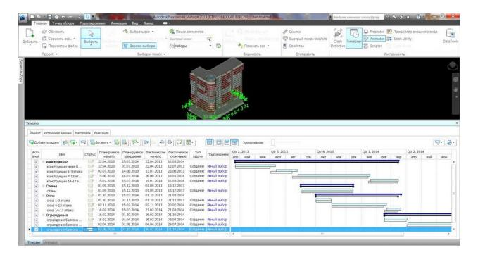
Figure 1. Schedule of construction of the building on the basis of the information model. Work in Revit Architecture and NavisWorks.
