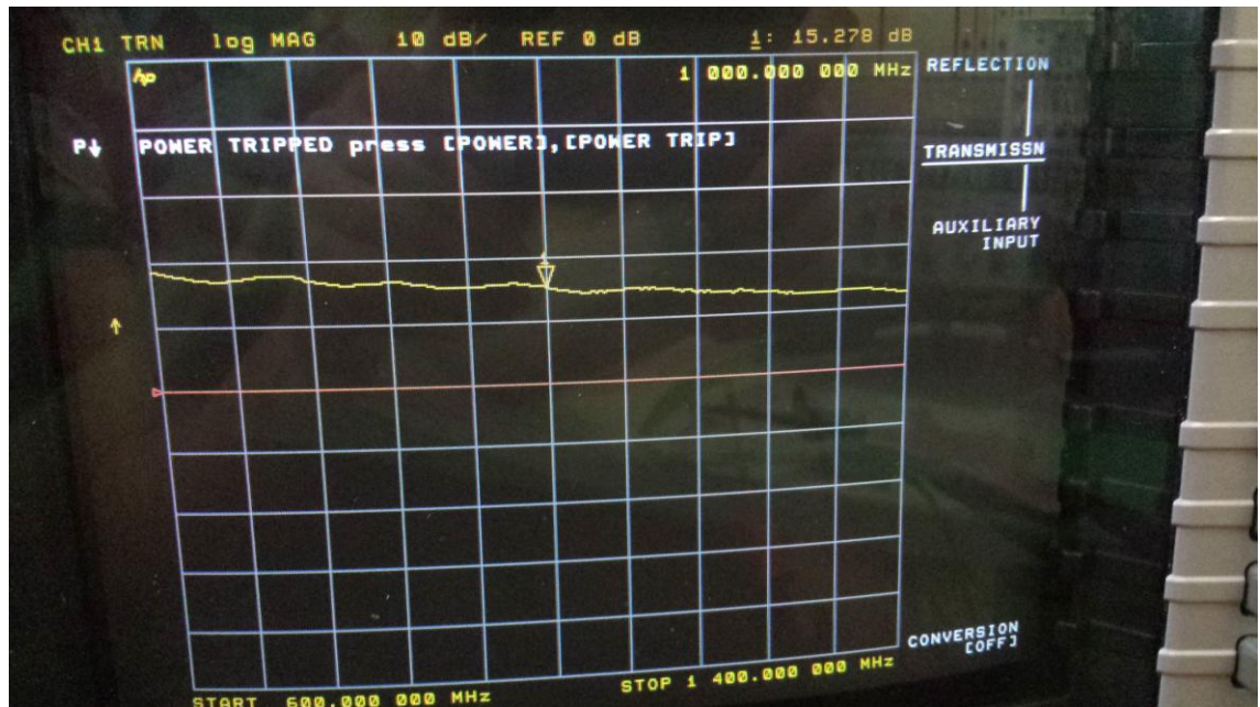
Figure 31. Gain graph as shown on the network analyzer screen
