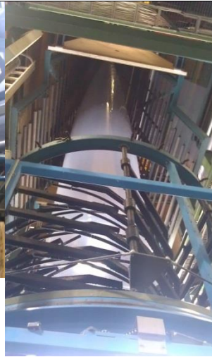
Figure 37 – Blown film is collected into sheet at the very top by the nip roll (image taken by author)
