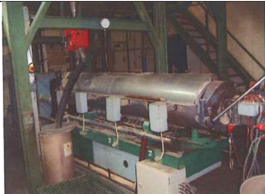
Figure 26 - Extruder's barrel (Hakkarainen, 2007), P. 28
