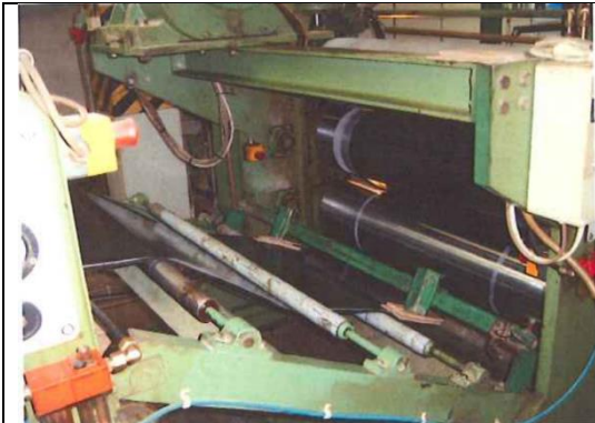
Figure 28 - Extruded resin is wound into rolls (Hakkarainen, 2007), P. 28
