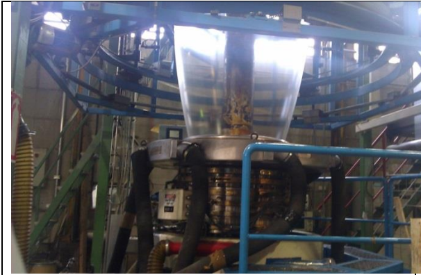
Figure 36 – Rotating blown film die (image taken by author)
