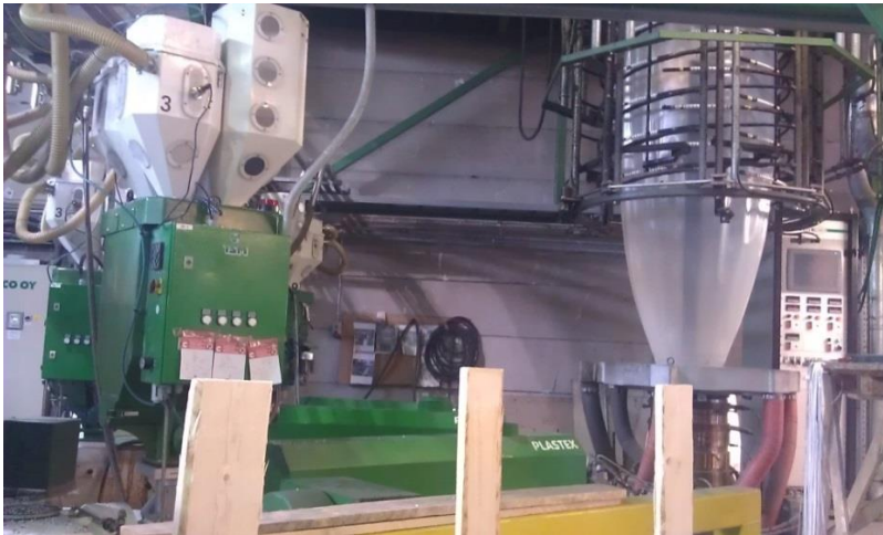
Figure 41 – Lamination film blowing process (image taken by author)
