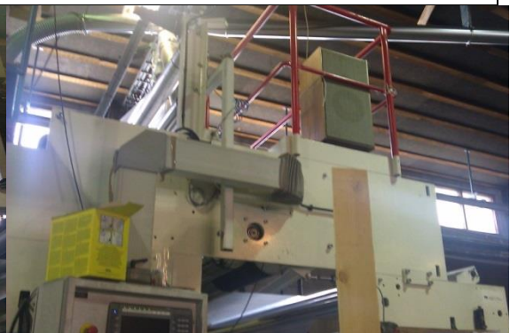
Figure 37 – Blown film is collected into sheet at the very top by the nip roll (image taken by author)
