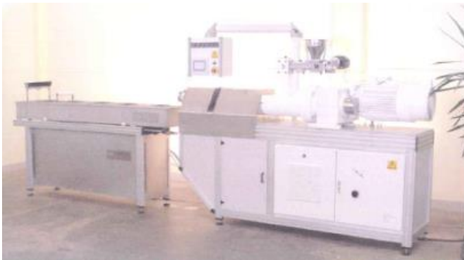
Figure 7 – Simple production line with extruder and cooling pool from KFM Machinery Ltd. (KFM, 2009)
