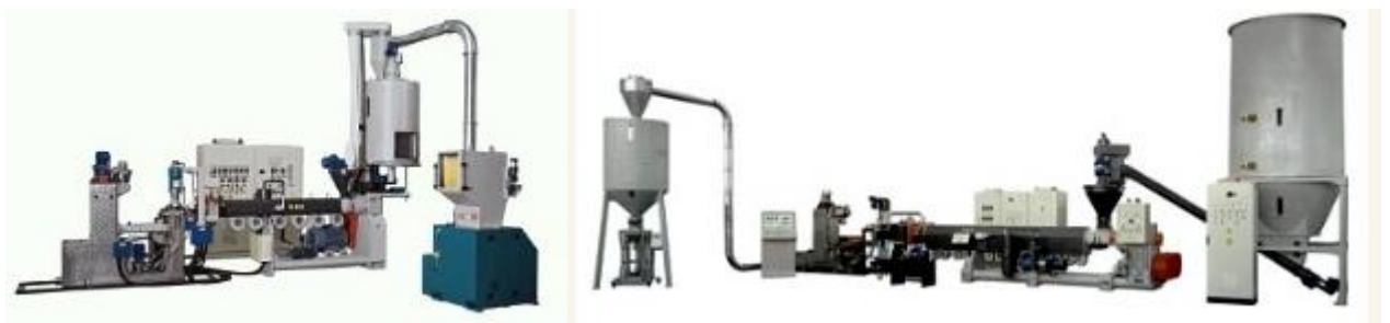
Figure 18- Recycling line and extrusion line of Tecnova s.r.l. (Cupton Oy, 2012)
