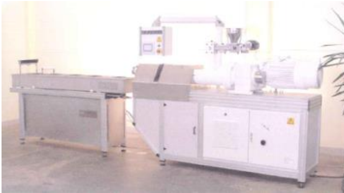
Figure 14 – Simple production line with extruder and cooling pool from KFM Machinery Ltd. (KFM, 2009)
