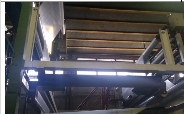
Figure 38 – Guiding rolls retracting the sheet from nip roll (image taken by author)
