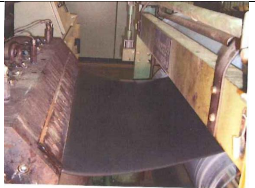
Figure 27 - Extruder's die and backwards rolling (Hakkarainen, 2007), P. 28
