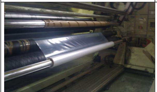
Figure 40 - Plastic film reeled in (image taken by author)
