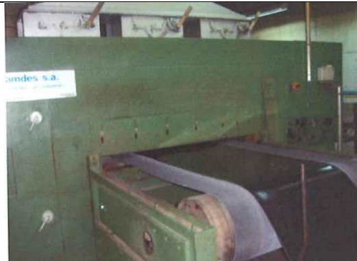
Figure 29 - The rolled resin is carried onto the furnace (Hakkarainen, 2007), P. 28
