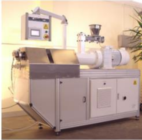
Figure 8 – KFM's Eco EX production extruder (KFM, 2009)
