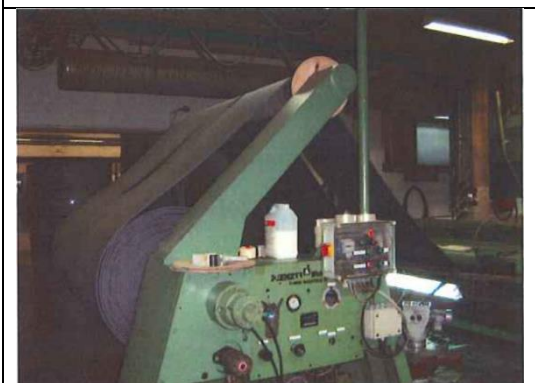
Figure 32 - Unwinding PE-X into rolls (Hakkarainen, 2007), P. 29
