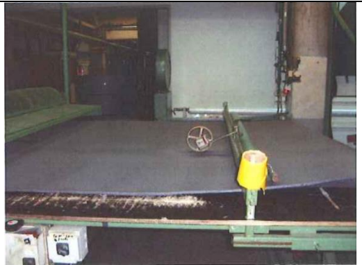
Figure 31 - Measurement wheel measures the length of the production batch, (Hakkarainen, 2007) P. 29
