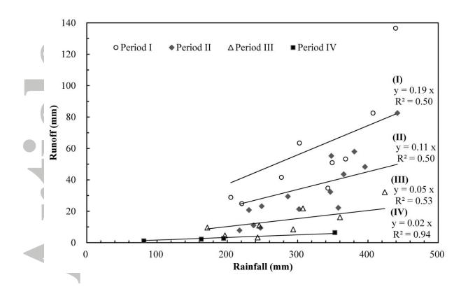
Figure 4 The linear regressions of runoff coefficients for the four periods in the HFC River basin.
