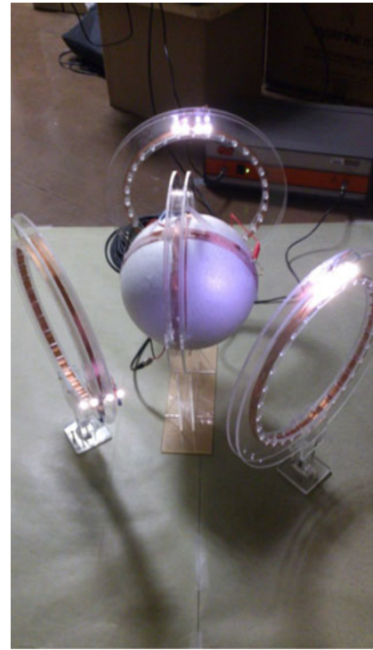
Fig. 5. Photograph showing that three LED loads are powered by three receiver resonators placed around a 2-D omnidirectional wireless power transmitter excited with two coil currents of the same magnitude but with a phase angle difference of 90^\circ .
