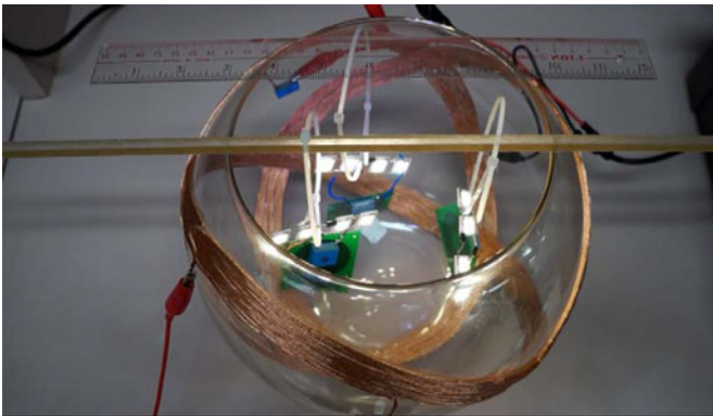
Fig. 9. Practical demonstration of the 3-D omnidirectional wireless power transfer system based on three excitation coils with angular displacements and the proposed nonidentical current control.
