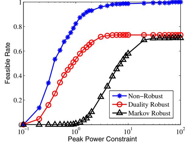
Fig. 7. The feasible rate of different methods with different peak power constraints.
