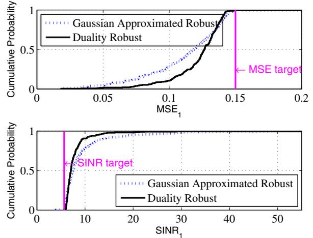
Fig. 5. The CDF of residual MSE and SINR for the proposed duality method and Gaussian approximated robust method.
