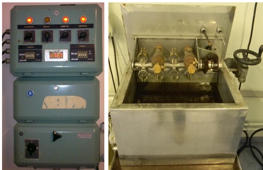
Figure 4.2 On the left hand side, control panel is illustrated and glycol bath is on the right hand side.
