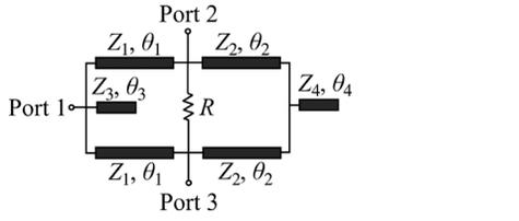
Fig. 1. Schematic of the proposed wideband bandpass power divider.
