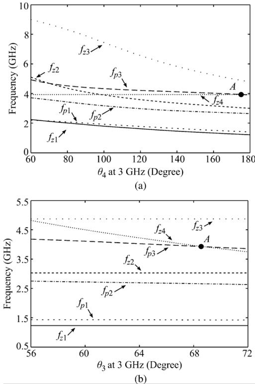
Fig. 3. Frequency locations of transmission poles and zeros versus electrical lengths of two open-circuited stubs. (a) When  $\theta_3 = 68.7^\circ$  at 3 GHz. (b) When  $\theta_4 = 176^\circ$  at 3 GHz. ( $Z_1 = 91.4 \Omega$ ,  $Z_2 = Z_3 = 115.1 \Omega$ , and  $Z_4 = 135.4 \Omega$ ).
