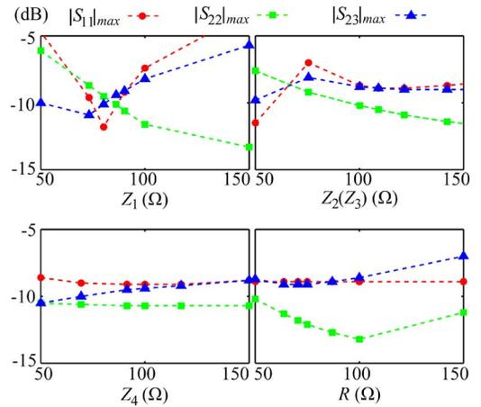
Fig. 5. Maximum reflections and isolations versus impedances ( $Z_i$ ) and loaded resistor ( $R$ ).
