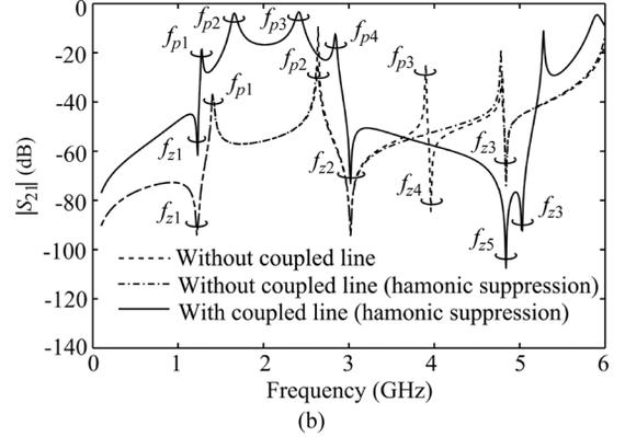
Fig. 4. Proposed power divider with coupled-line sections. (a) Schematic. (b) Frequency responses of S-magnitudes under the weak coupling.
