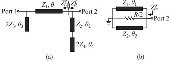
Fig. 2. (a) Even-mode circuit model. (b) Odd-mode circuit model.
