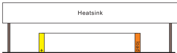
Fig. 5. A microstrip line structure with a heatsink on top of it.
