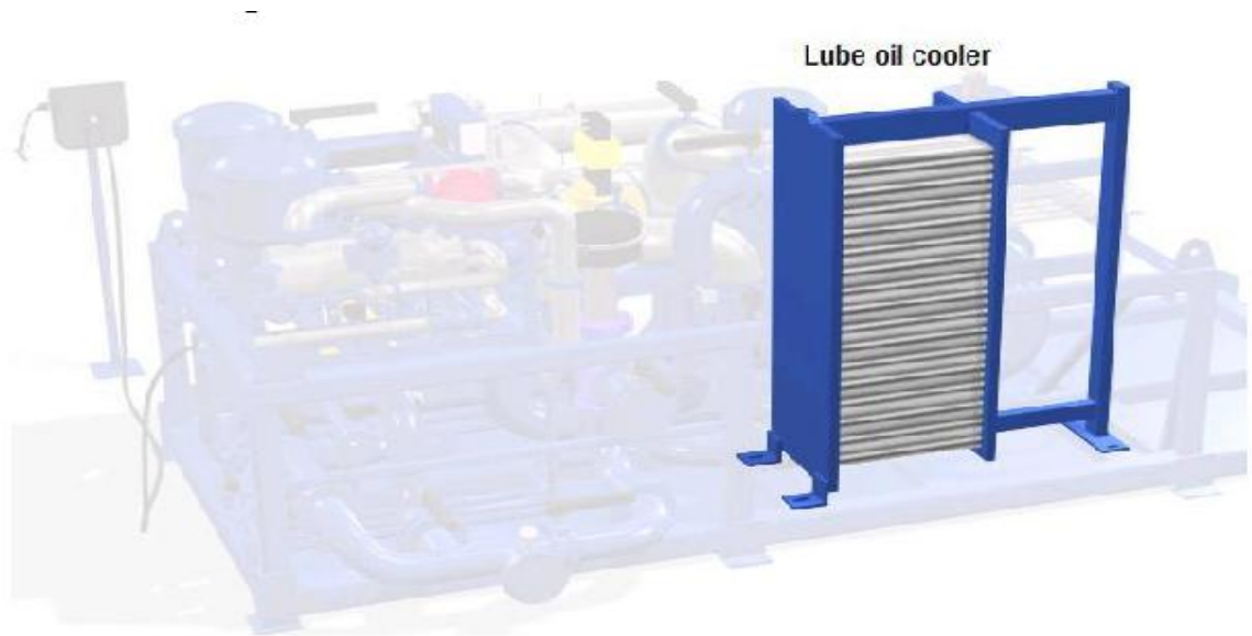
Figure 9. Lube oil cooler as a heat exchanger. /3/
