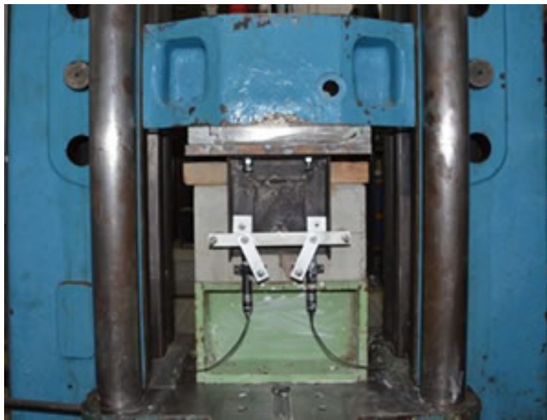
Figure 8. Bolt test set-up for the “HIT-RE 500 + HAS-E” anchoring system; (a) design diagram and (b) actual arrangement (dimensions in millimeters)
