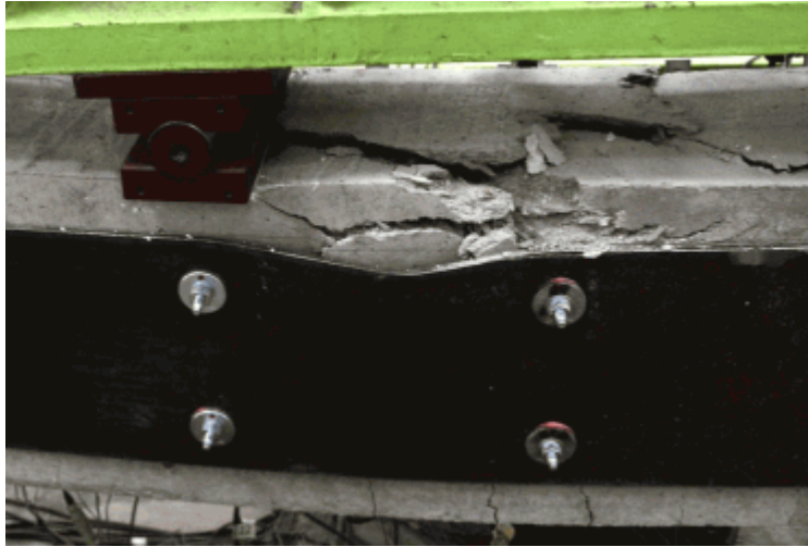
Figure 16. Plate buckling of Specimen P250B300
