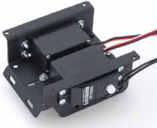
Figure 9: Step 2 - Servos' installation [11]
