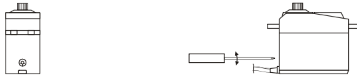
Figure 24: Servos' set point adjustment screw [9]
