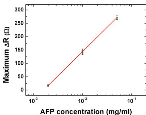
FIG. 5. (Color online) Plot of maximum  $\Delta R$  vs AFP antigen concentration. The error bars represent the standard deviations for the  $\Delta R$  between 30 Oe and 50 Oe. The fitting curve (solid line) illustrates that  $\Delta R$  changes logarithmically with the concentration of target AFP antigens.
