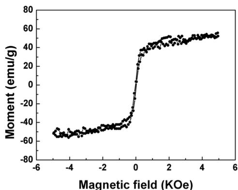
FIG. 1. VSM measurement showing the magnetic moment as a function of applied magnetic field. The samples of the iron-oxide MNPs with carboxyl groups were measured in the solvent of DI water. The saturation magnetization is 50 emu/g.
