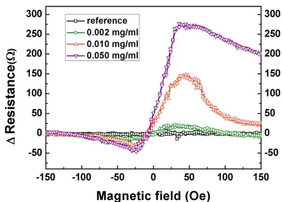
FIG. 4. (Color online) Diagram of the MTJ sensor resistance variations  $\Delta R$  after binding with three different concentrations of target AFP antigens. The maximum resistance deviations appear at approximately 40 Oe, with the maximums of 17, 143, and 271  $\Omega$ , respectively.
