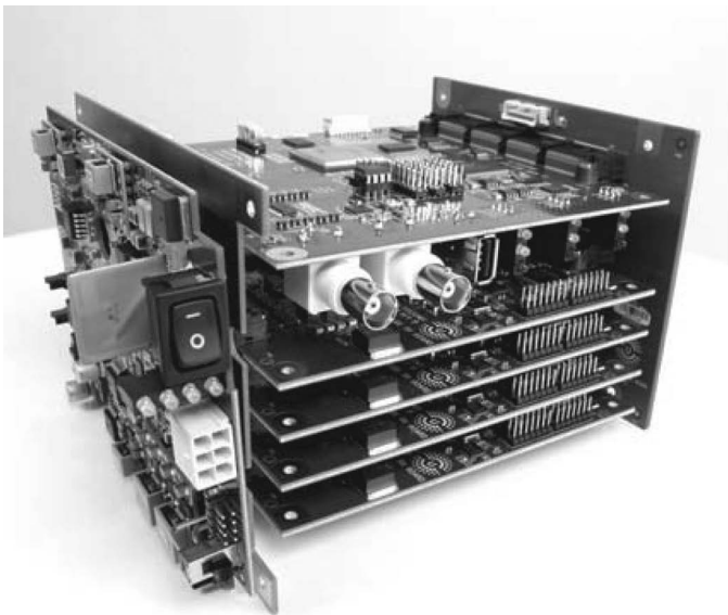
Fig. 2. Photo of the multi-channel pre-beamformed data acquisition (DAQ) system. The four horizontally aligned boards at the bottom of the picture are the receiver boards (each responsible for DAQ over 32 channels); the one at the top is the main controller board. The left and right boards are, respectively, the power module and the connector board.
