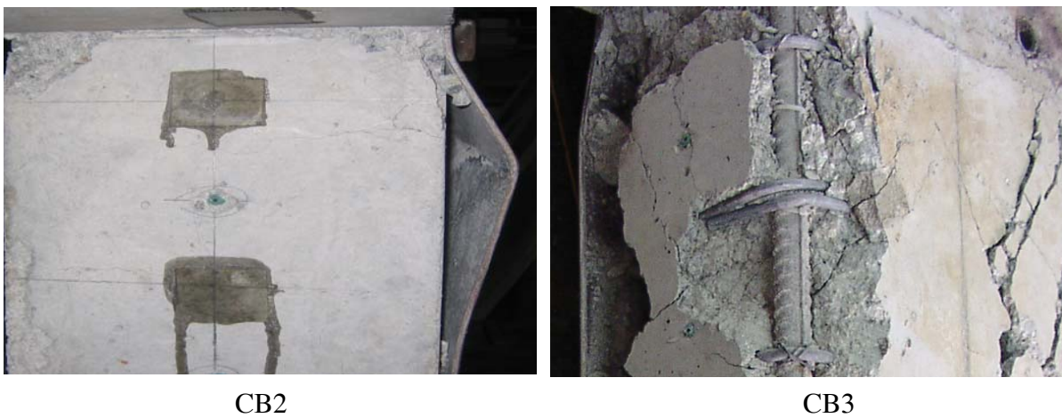
Figure 11. Local Buckling of Specimens at Failure Stage
