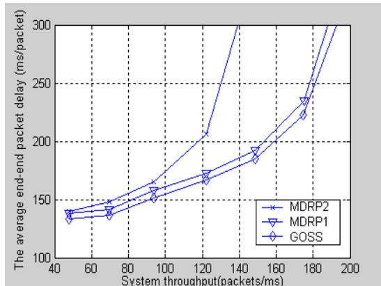
Fig. 10: performance comparison of GOSS and MDRP (unidirectional traffic)
