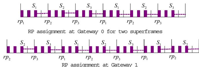
Fig. 3: RP assignment for scatternet in Fig. 1 using GOSS
