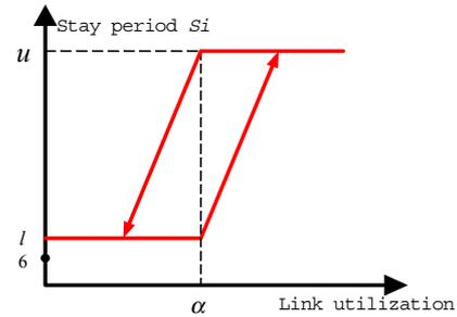
Fig. 6: adapting stay period based on link utilization.
