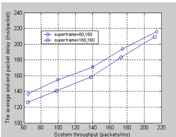
Fig. 12: degree-based superframe against common superframe (unidirectional traffic)
