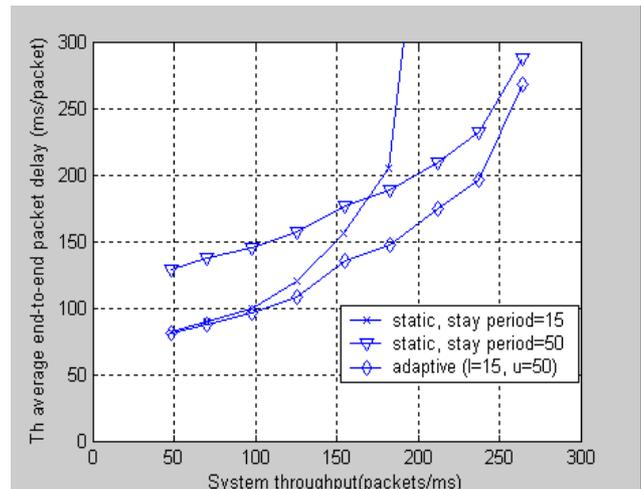
Fig. 13: adaptive GOSS versus static GOSS
