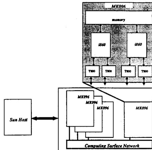
Figure 2: Block diagram of Meiko™ Computing Surface
