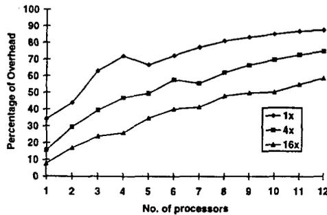
Figure 10: Percentage of overhead on median filtering
