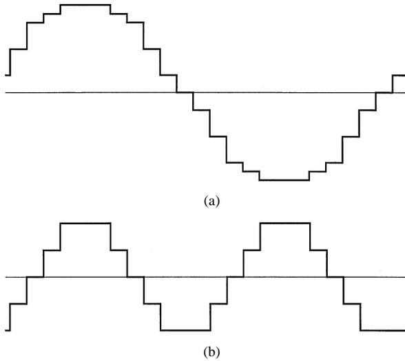
Fig. 2. Pole-changing MMF waveforms. (a) Two-pole. (b) Four-pole.
