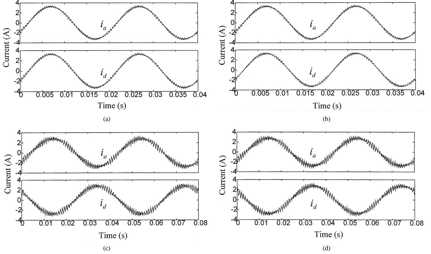
Fig. 5. Simulated current waveforms. (a) 4P1. (b) 4P2. (c) 2P1. (d) 2P2.
