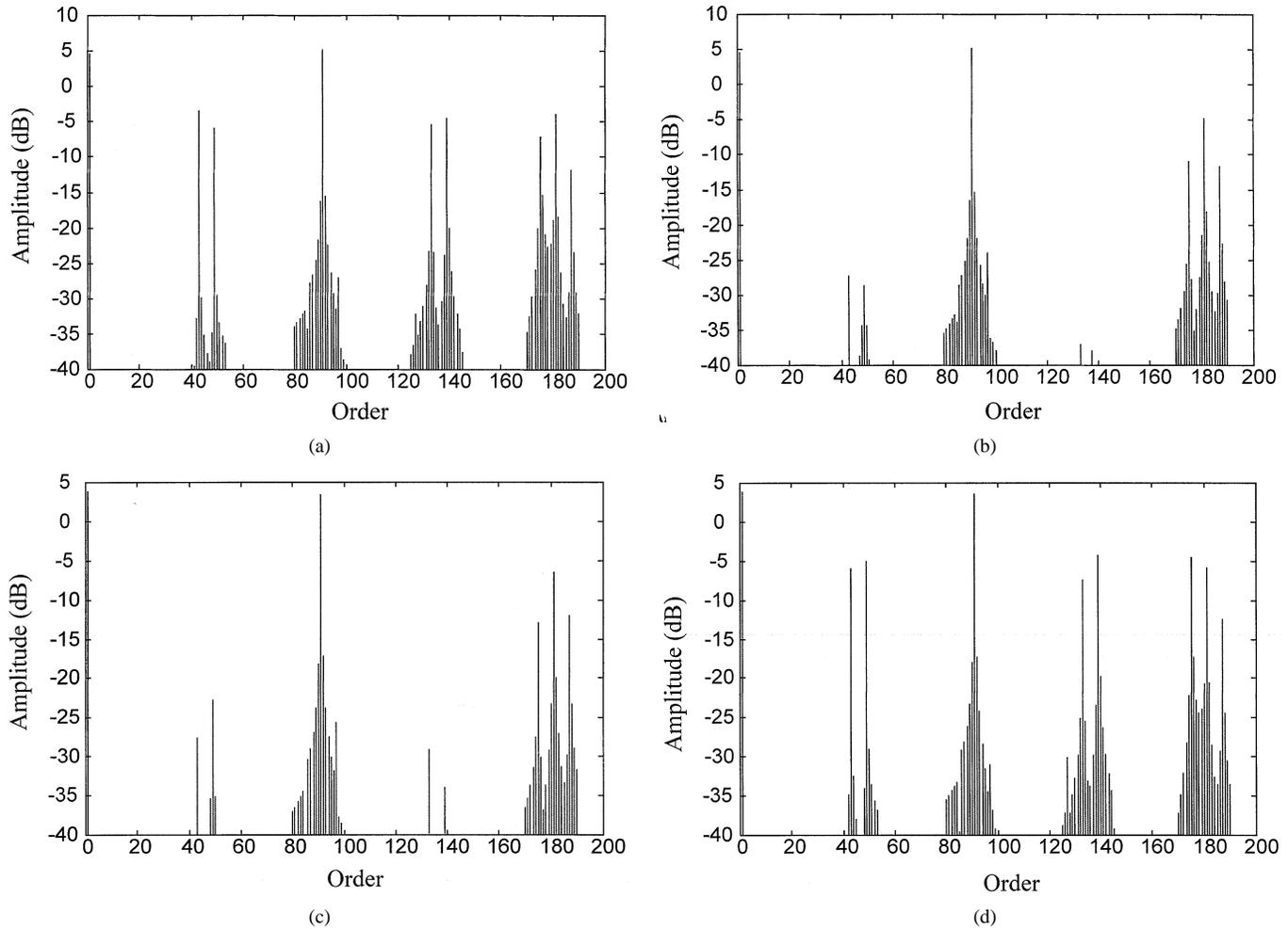
Fig. 7. Simulated current spectra of dc link. (a) 4P1. (b) 4P2. (c) 2P1. (d) 2P2.
