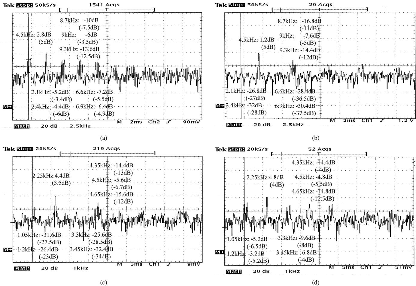
Fig. 11. Measured current spectra of dc link. (a) 4P1. (b) 4P2. (c) 2P1. (d) 2P2.
