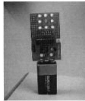
Fig. 25. The 8-LED transmitter prototype (constantly illuminating and transmitting information).
