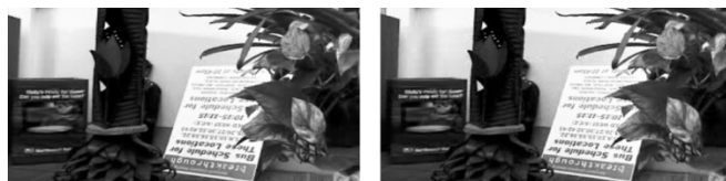
Fig. 14. Rendered views of the concentric mosaic Lobby after decompression: (a) using the normal setup sequence (compression ratio: 65.28; mean PSNR: 35.72 dB) and (b) using multiperspective panoramas (compression ratio: 42.01; mean PSNR: 34.50 dB).
