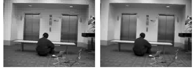
Fig. 17. Decompressed B -pictures using: (left) the modified MPEG-2 algorithm (compression ratio: 175.12; mean PSNR: 30.78 dB) and (right) the proposed subsampling compression scheme (compression ratio: 171.26; mean PSNR: 30.27 dB).
