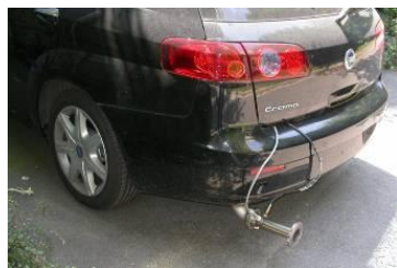
Figure 8: SrFe 0.6 Ti 0.4 O 3 sensor prototype equipped on a Fiat Croma exhaust line.
