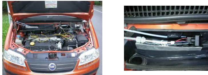
Figure 10: \text{In}_2\text{O}_3 sensor prototype equipped on a Fiat Idea cabin inlet air duct
